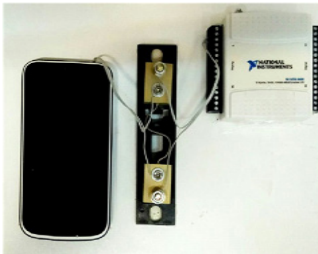
(a) Mobile energy measurement hardware.
